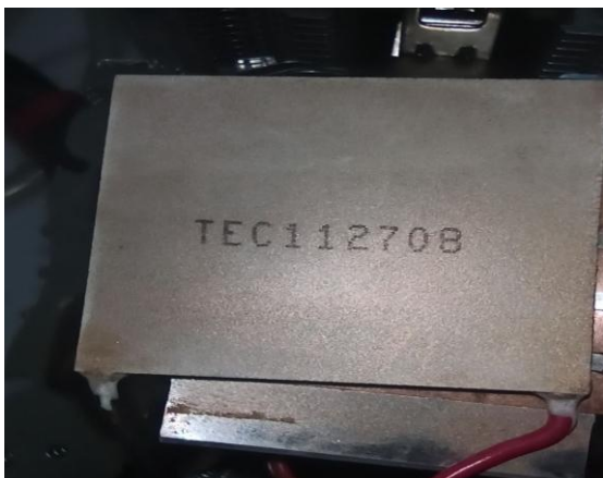
Figure 7: Thermoelectric cooling chip
