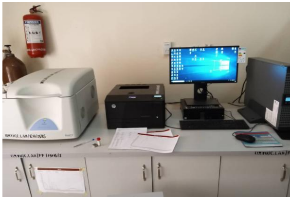
Figure 6: TGA Apparatus 4000 BY Perkin Elmer
