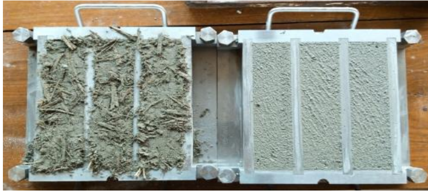
Figure 9 : Molding of test pieces
