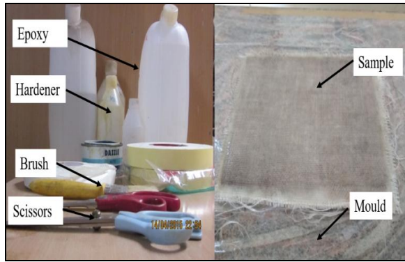
Fig. 1 Hand layup process
