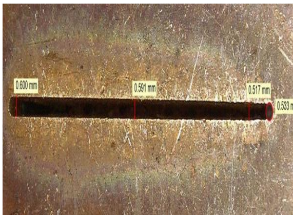
Figure 5: Kerf Width Measurement
