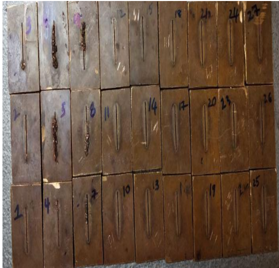
Figure 4: 27 Pieces After Machining on Single Piece
