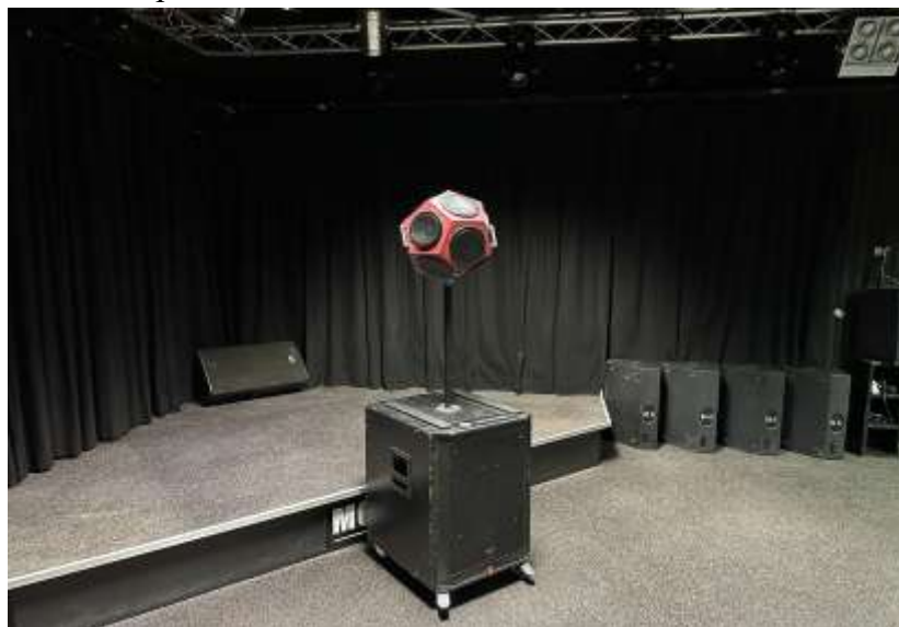
Figure 1: Omnidirectional dodecahedron loudspeaker mounted on a subwoofer, used as the sound source in the concert hall.
