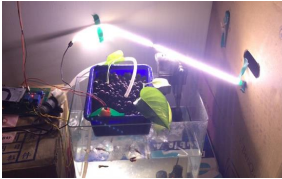
Figure 15: System Auto-Sensing Lighting
