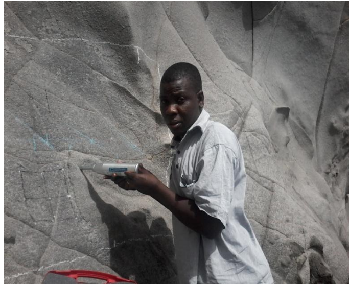
Figure 3. In situ Schmidt hammer rebound testing for the geomechanical characterization
