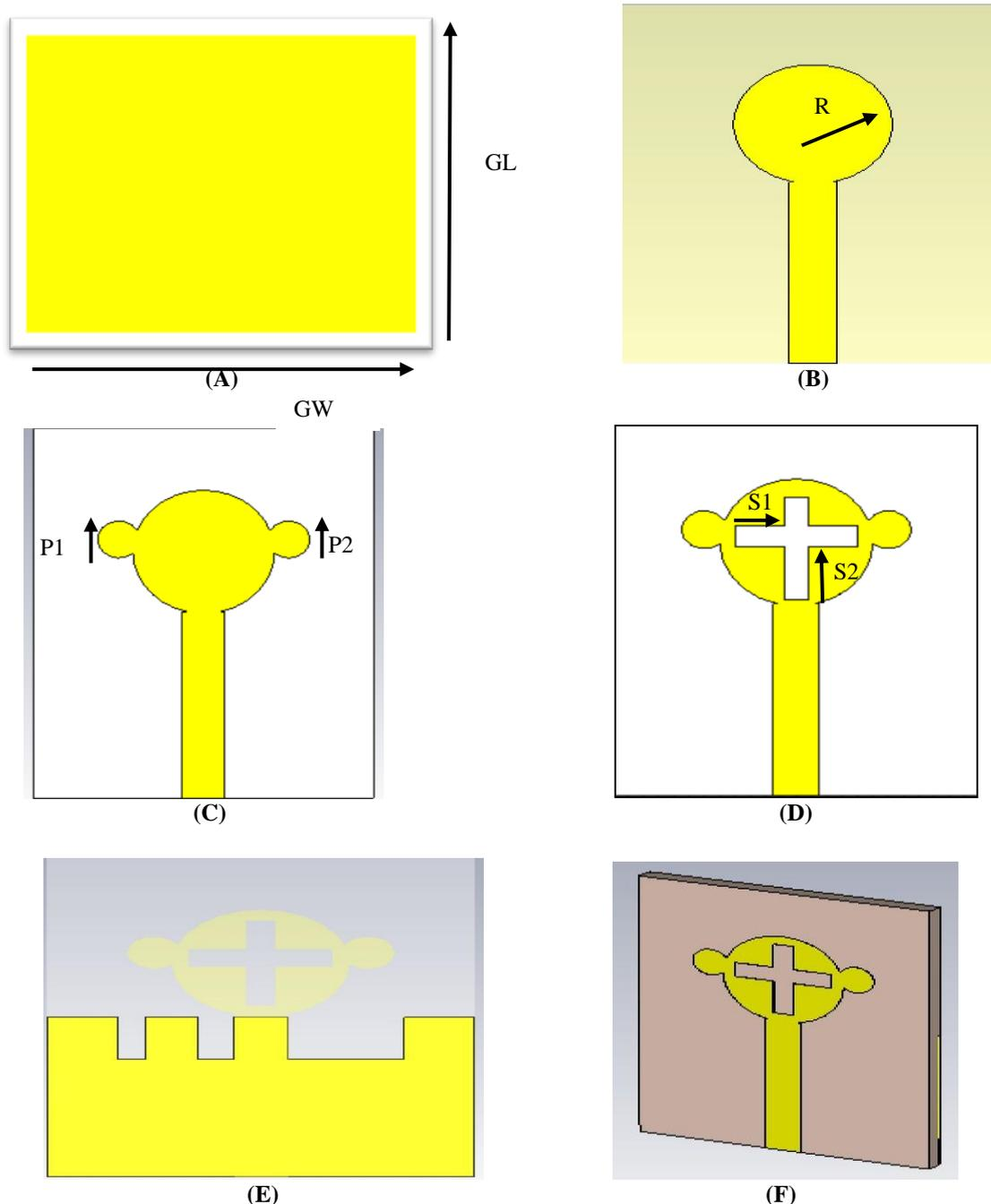
**Figure 1: Evaluation of Proposed antenna at Different phases (A) ground plane (B) Circular patch (C) Patch with Stubs (D) patch with stubs and slots (E) Ground plane with slots (F) Perspective view**
