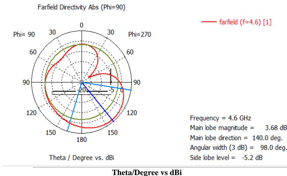
**Figure 5 Radiation Pattern of Port 1 at 4.6Ghz**
