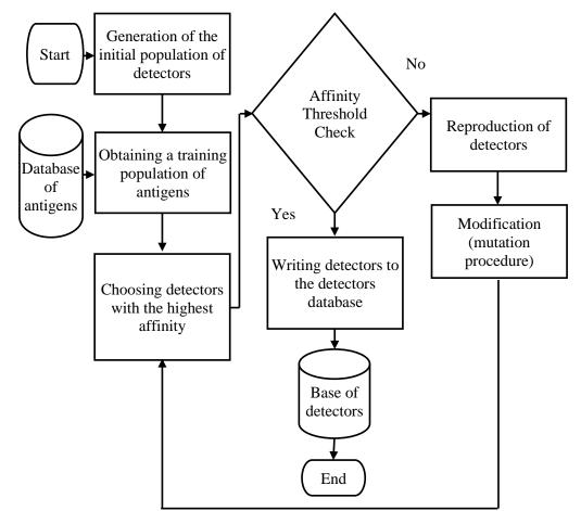
Figure 1. Scheme of generating detectors by the clonal selection algorithm of the artificial immune system for detecting suspicious activities
