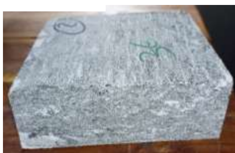
Fig. 3 : Sample of rock cut by non-destructive testing (Sclerometer and ultrasound)
