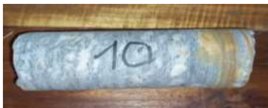
Fig. 1 : Core rock sample for uniaxial compression testing
