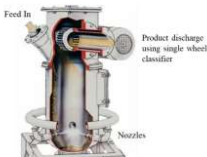
Figure 7: Schematics of a fluidized bed opposed jet mill.
