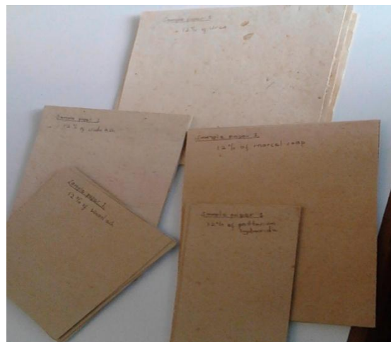
Figure 1: Photo of handmade papers samples made from rice straws using various delignifying agents.
